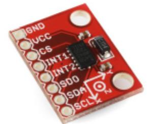
The ADXL345 is well suited to measures the static acceleration of gravity in tilt-sensing applications, as well as dynamic acceleration resulting from motion or shock. Its high resolution (4 mg/LSB) enables measurement of inclination changes less than 1.0 degrees;
