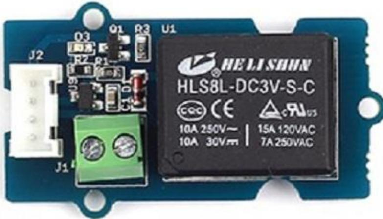
The Grove-Relay module is a digital normally-open switch. Through it, you can control circuit of high voltage with low voltage, say 5V on the controller. There is an indicator LED on the board, which will light up when the controlled terminals get closed.
