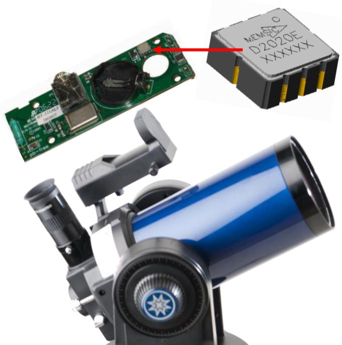
**Note:** The MEMSIC logo's arrow indicates the  $+X$  sensing direction of the device. The  $+Y$  sensing direction is rotated  $90^\circ$  away from the  $+X$  direction.
