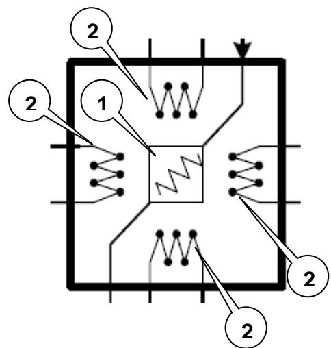
Acceleration in any direction will disturb the temperature profile, due to free convection heat transfer, causing it to be asymmetrical. The temperature, and hence voltage output of the four thermopiles will then be different. The differential voltage at the thermopile outputs is directly proportional to the acceleration. There are two identical acceleration signal paths on the accelerometer, one to measure acceleration in the x-axis and one to measure acceleration in the y-axis.
