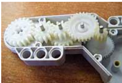
Close-up on the gear train. From motor to output shaft, we get these gear ratio:
