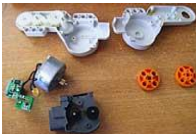
Exploded view of the motor.
