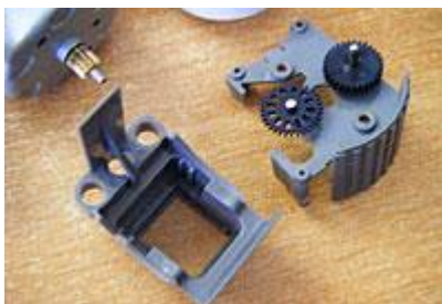
Encoder wheel and enclosure back parts. We have 12 slits in encoder, and motor to encoder gear reduction is 10:32. So for 1 turn of output hub, encoders turns 48 \cdot 10/32 = 15 turns, optical detectors sees 15 \cdot 12 = 180 slits. Using both sides of slits gives nominal 360 ticks per turn resolution. Note that since we have a quadrature encoder, the maximum resolution is 720 ticks/turn, but this is not used by standard NXT firmware.
