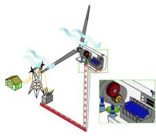
A tall tower is built with a propeller on the top. The wind blows the propeller round, which turns a generator to produce electricity
